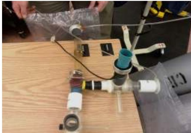
Figure 7. Photograph of the equipment set-up for hypothesis 2 testing for the 2 L compliant mixing bag.
